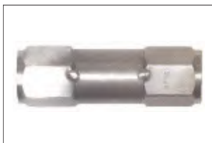
Tacked ends to prevent accidental removal of end connectors.
